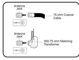
Connect the 75 ohm cable from the combination VHF/UHF antenna to the antenna jack.
